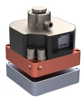
The Focus Beam Profiler FBP-1KF is a robust and compact analysis system to measure a focused laser with up to 400W power. The FBP-1KF is based on a multi-stage high-performance attenuator.
